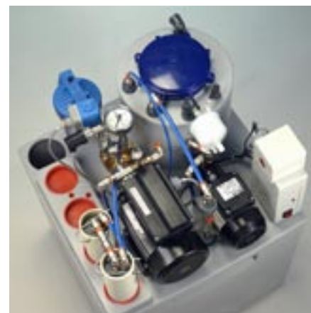
The reservoir pump supplies a stable flow of 250 litres per hour at 1.5 bar pressure.
